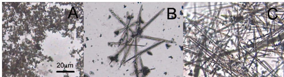
Fig. 4. Morphology of the hydrothermal products at 165 °C for different times of (A) 20, (B) 30, and (C) 40 h. Reproduced with permission from [60], X. Ding et al., Hyperbranched Polymer-Assisted Hydrothermal In situ Synthesis of Submicrometer Silver Tubes. Crystal Growth & Design 8, 2982 (2008).
